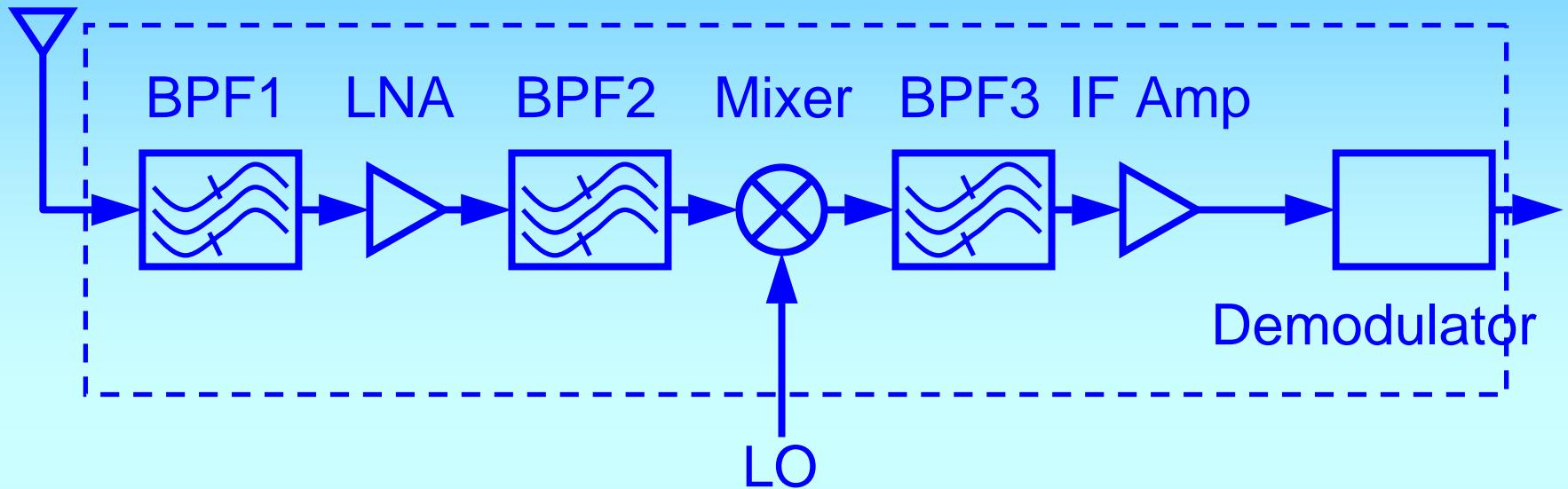
RF Receiver, DUT (Device under Test)
